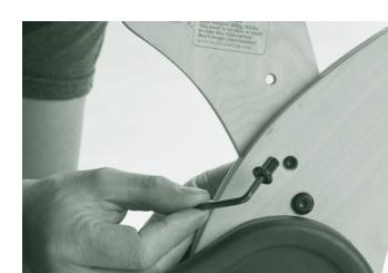
1. Insert seatpost bolt and tighten the capping nut. Repeat.
