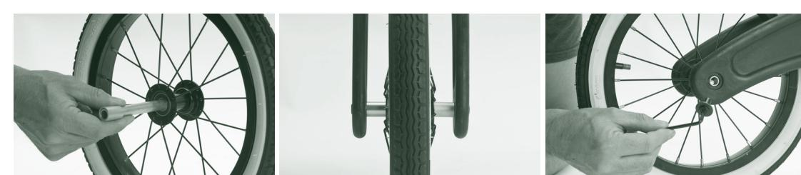
1. Insert axle tube through rear wheel hub. Thread mini spacers on each end.
