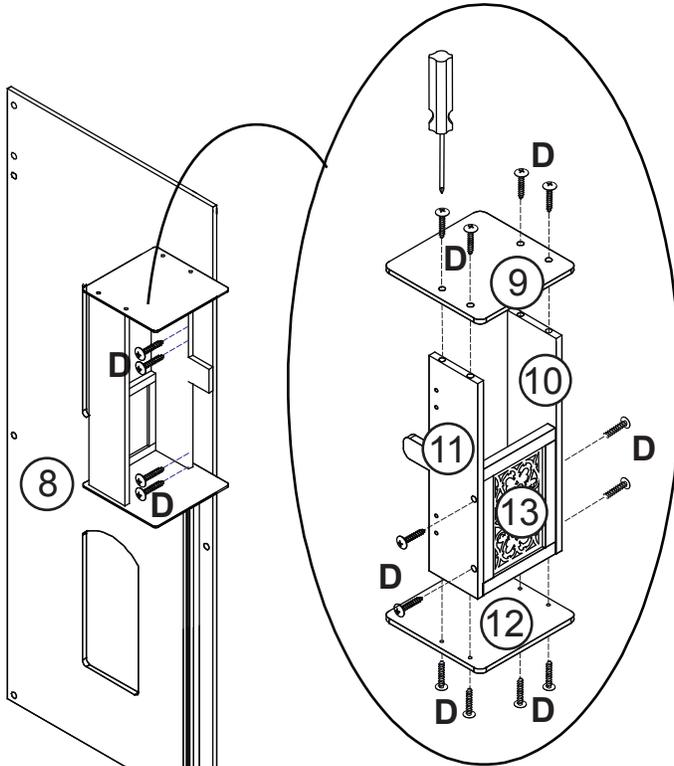
Wait to assemble part 10 until after elevator is assembled to the track pieces.
